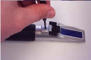
Turn the calibration screw (see photo at left) until the boundary between the upper blue field and the lower white field meet exactly at ZERO on the scale.
