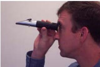
Hold the refractometer in the direction of a natural light source and look into the eyepiece. You will see a circular field with graduations down the center. You may have to focus the eyepiece to clearly see the graduations. Figure 1 (below) shows what you would see if you looked through the refractometer without any sample present.
