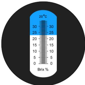
As you can see from this sample of Barleywine the reading is 23% Brix. This can be quick converted using the rule of 4 to 1.092 or exactly with the chart to 1.097.
