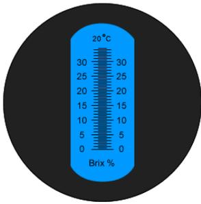
you are using natural light to view the readings; you should not read a refractometer in the presence of fluorescent light.
