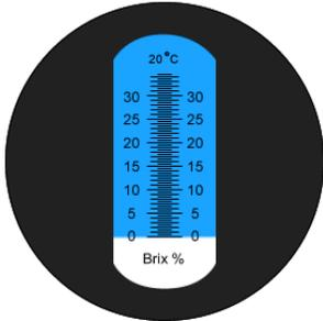
Notice that the reading is taken where the blue and the white meet. Calibrate to ZERO using distilled water as the sample.
