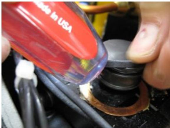
Then slide the seal into place over the O ring. This can be a little tricky as it is a very tight fit; it may help to use the handle of a screwdriver to nudge the seal into place.
