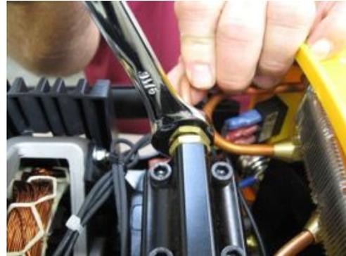
Carefully lift up the top of the cylinder head exposing the valve plate and base. If it is evident that the valve itself is melted (See photo below), be sure and check the fan and fan gear box assembly. If that failed, replace the gear box only (Part# AY0030) or the fan and gear box assembly (AY0030c).
