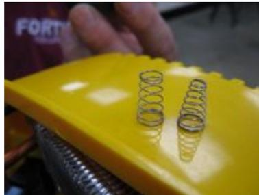
The smooth side of the valve plate is inserted into the top of the cylinder head. Feed the valve with the head through the valve plate and thread the spring with the smaller opening over the head of the valve.
