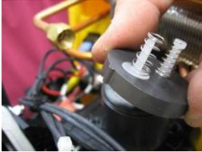
Slide the cylinder head over the valve plate, insert the four Allen bolts and start to thread them in. Use the removable type thread sealant and tighten the bolts making sure the cylinder head is evenly secured. Reinstall and tighten the flair nuts.
