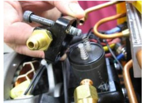
Carefully lift the cylinder from the compressor block. Note the camber on the bottom of the cylinder, this end will need to go down when reassembling the machine. Also note the copper shim; this will also need to be in place for reassembly.
