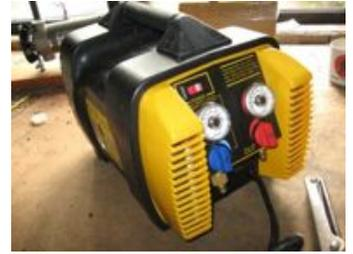
After years of pumping liquid refrigerants, components wear. To check the performance of your G5 Twin, disconnect any hoses and **double check the inlet screen to be certain it is free of debris**. Open both valves wide open and turn on the machine. Close the output valve and time how long it takes to shut off on the high pressure switch (should be about 550psi).
