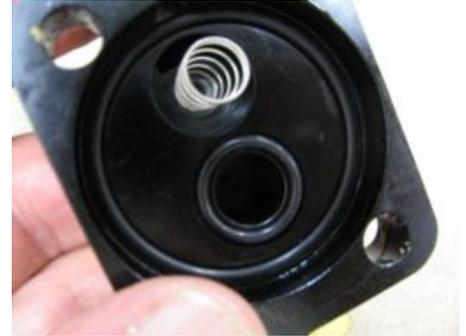
You can now install the new valves. Note the two different types of springs included in the rebuild kit.
